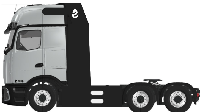
Europa Series Edition - 6x2: 5th wheel load: 12-16.5 tonnes (depending on configuration)
