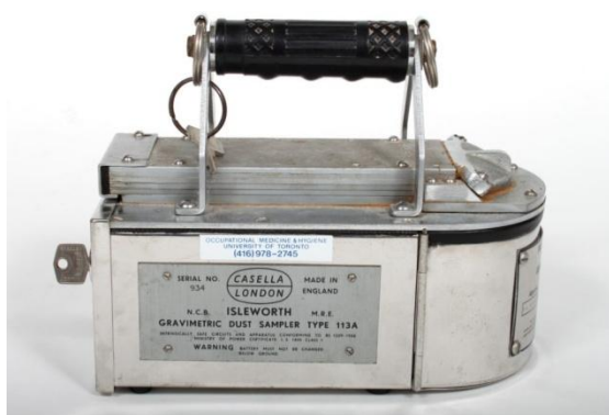
Fig 8.4. The MRE gravimetric dust sampler. The dusty air is sucked through a stack of parallel plates (the “elutriator”) designed to select according to the MRC respirable definition (Fig 8.3). Photograph by courtesy of the University of Toronto Scientific Instruments Collection https://utsic.utoronto.ca/
