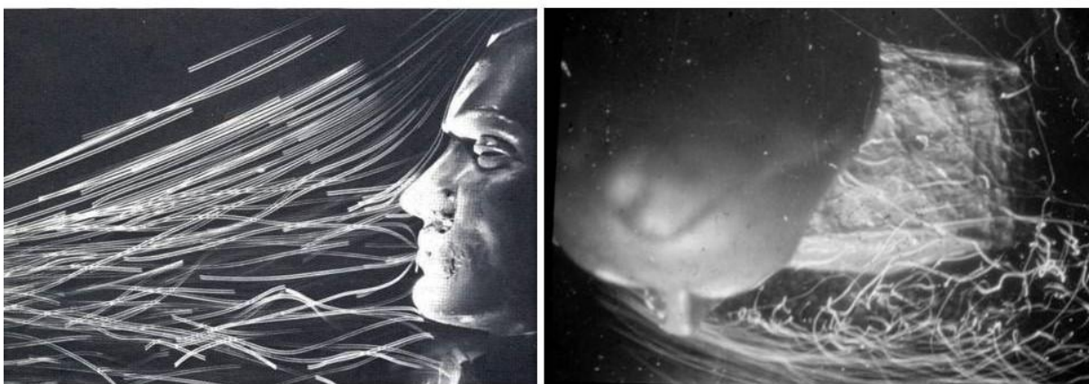
Fig 8.5 The flow past a model head inhaling steadily through the mouth at 40 litres/min, facing and side-on to a wind of 0.7 m/sec. The flowlines are made visible by neutral-density helium-filled soap bubbles. Particle inertia makes the particles cross the flowlines where they curve, and this affects the “inhalable” concentration. (Right-hand photo courtesy of Institute of Occupational Medicine)
