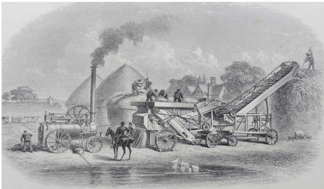
Fig 3.3. Top, Garrett's threshing machine, about 1867. The sheaves are fed in on the top of the machine, at the left end. The heads of grain come into the sacks below and the straw is ejected top right. A similar machine is seen in operation in the lower picture, with a mobile steam engine providing the power. The process here looks clean, but a lot of dust would have been ejected with the straw, and with the grain. Top picture from the National Encyclopedia (1867) and the lower from The Popular Encyclopedia (about 1875)
