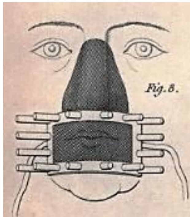
Fig 1.4. Abraham's magnetic "muzzle", for protecting needle grinders. A wooden frame holds "two or three thicknesses of crape or muslin, and is studded with 16 magnets". The cloth is held over the nose by bent wire. The magnets are intended to collect much of the iron dust before it reaches the cloth. Illustration from
