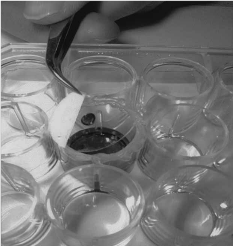
Fig. 2. Hanging-drop vapor-diffusion setup in 24-well tissue culture plates.
