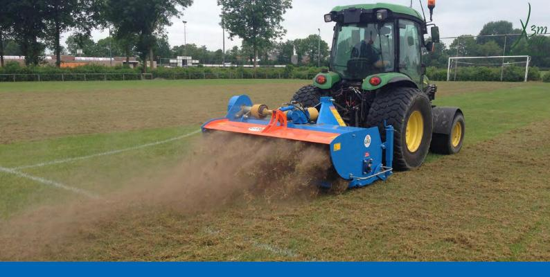
Because of our patented roller pendulum system you are easily in control of the operating depth. As a unique bonus, we have provided the scarifying machine with a hydraulic adjustable slide. This is ideal when you are required to scarify near the edges and corners of a pitch. Consequently, swiping and cleaning of soiled advertising boards and pathways are history.
