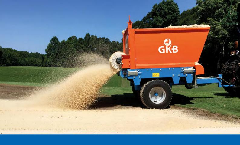
Since the brush is hydraulically powered, the quantity of material applied can accurately be determined.
