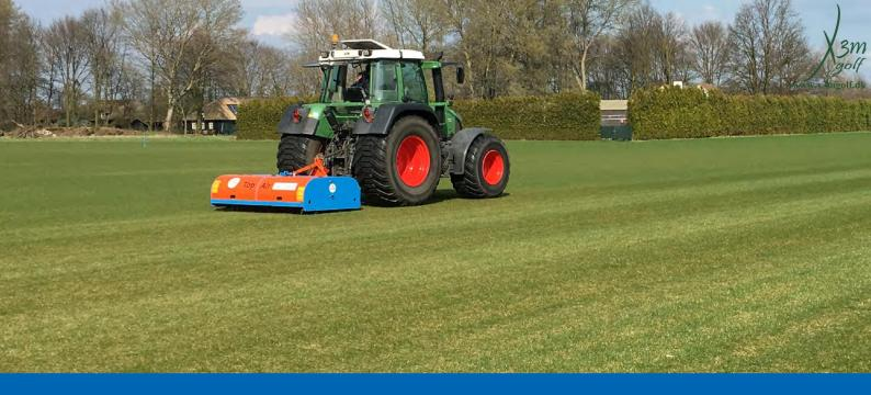
Finally, it is also possible to combat against white grubs when you assemble cutting blades instead of the Evolvente® blades. The combination of operations contributes to the reduction of the CO2 emission and the process of chemical free management of your sports pitch.
