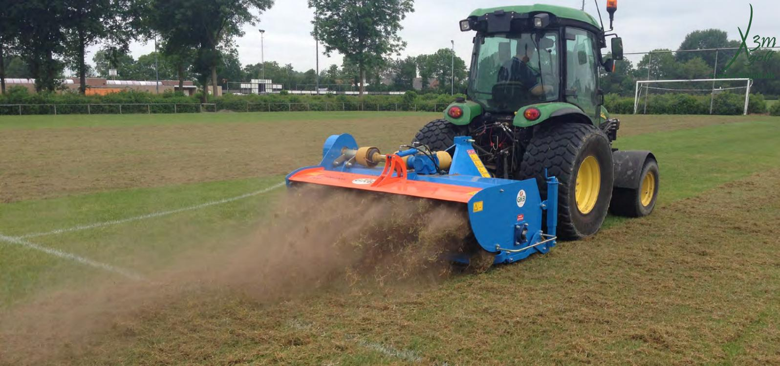
Because of our patented roller pendulum system you are easily in control of the operating depth. As a unique bonus, we have provided the scarifying machine with a hydraulic adjustable slide. This is ideal when you are required to scarify near the edges and corners of a pitch. Consequently, swiping and cleaning of soiled advertising boards and pathways are history.
