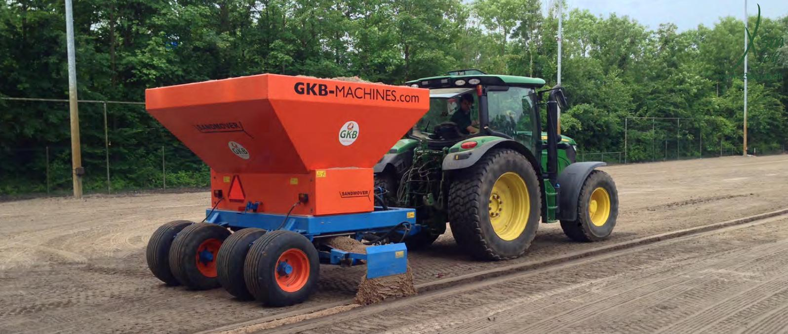
The Sandmover rests on four broad balloon tyres, to minimize the risk of possible damage on the pitch. Optionally, you can choose a design in which the machine will rest on radial balloon tires and we can provide the outer wheels with hydraulic brakes. Additionally, you have the option of selecting a trench filler and conveyer belt.
