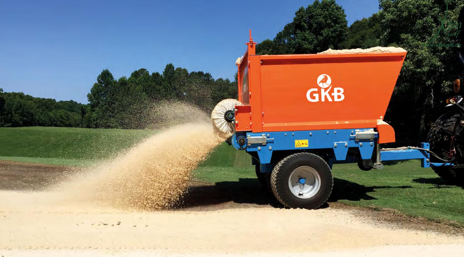
Since the brush is hydraulically powered, the quantity of material applied can accurately be determined.
