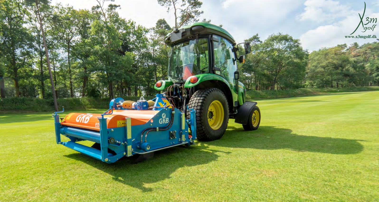
You can level imperfections in your pitch by carrying the recycled dressing soil on the conveyer belt, following you can scatter it on the desired area of the pitch.
