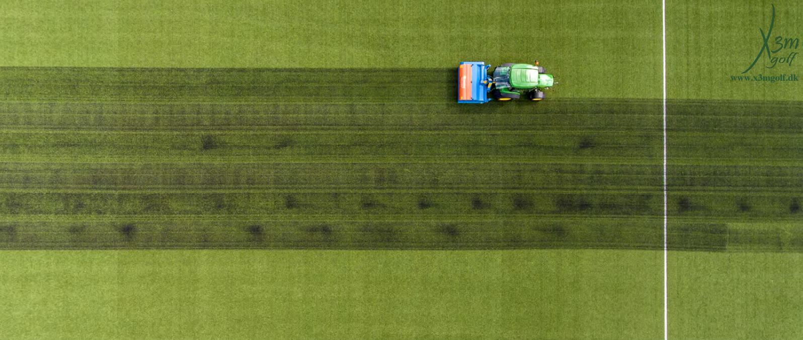
The synthetic turf brush will brush the infill material with all the contamination that it is containing and will cast it on a vibrating screen. Depending on the type of pitch that you are cleaning, you attach one of the three types of screens (rough to fine). The coarse dirt will be moved to the collection container, dust and other lightweight dirt will be absorbed by a suction unit with a dust bag.
