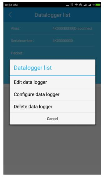
There are 3 options in the dialog window, "Edit data logger" is used to assign alias for the WiFi-E module; "Configure data logger" is used to configure the connection of WiFi-E module to router; "Delete data logger" is used to delete the WiFi-E module.
