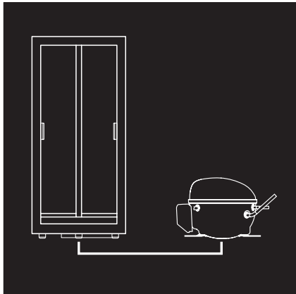
REMOTE REFRIGERATING UNITS
