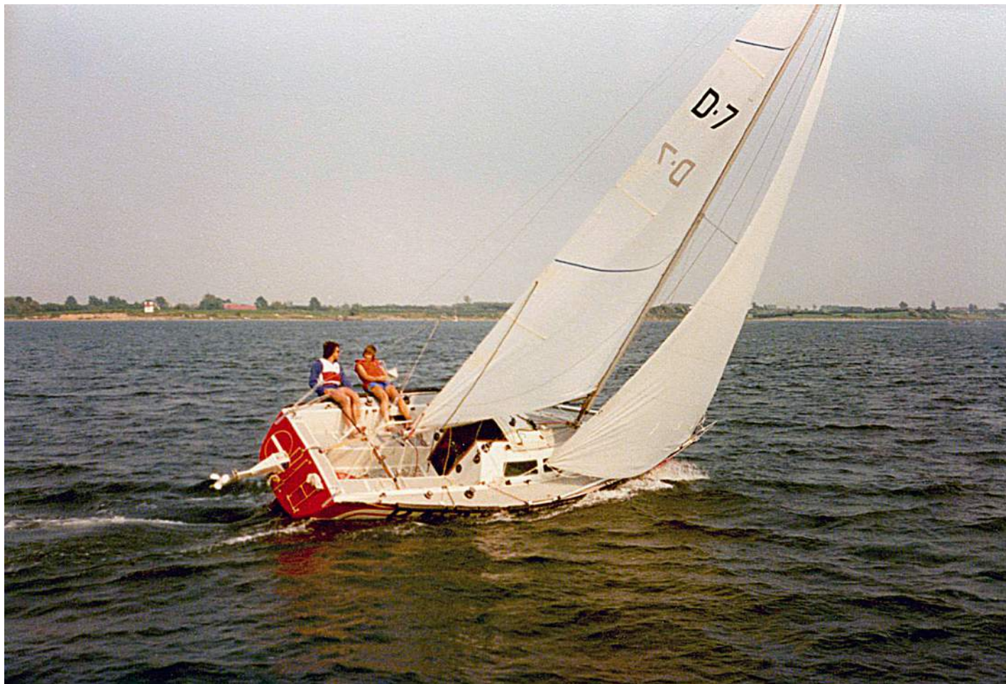
Niels' first design, the prototype for Banner 30, was the Banner 29. It had an outboard engine fitted to the sliding transom bracket
