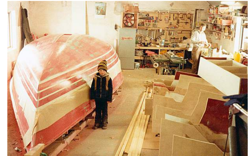
X-79 hull plug almost ready for the final finish before the lines are applied. It is Lars Jeppesen to the left.
