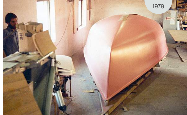
X-79 hull plug almost ready for the final finish before the lines are applied. It is Lars Jeppesen to the left.
