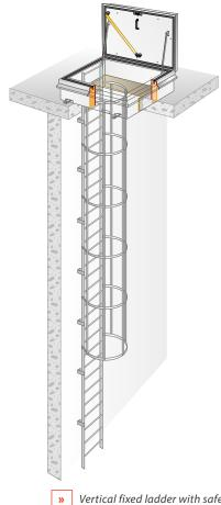
Fixed ladders are supplied with a pre-assembled cage with five strips (cage if applicable) and ladder supports for fixing to the external wall of the building.
