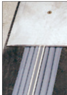
Installation is completed with aluminum or stainless steel coverplates. The center spline functions as a continuous receptor for the self-locating coverplate screws allowing for greater ease of installation. The coverplate edge-chamfer is available in standard or optional low-slope configurations.
