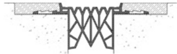
Thermaflex is constructed of extruded thermoplastic Santoprene® rubber sealing glands with punched flanges embedded in a high-strength, flexible, impact-absorbing elastomeric nosing.
