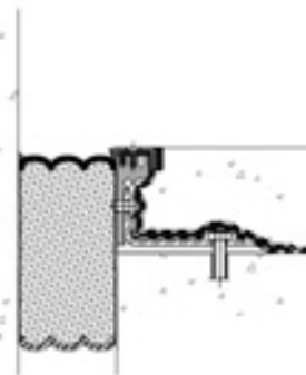
DFR-FP is an effective fire-rated watertight expansion joint which can bridge split-slab to solid-slab construction. The connection to solid-slab construction is made directly to the slab substrate. The split-slab connection is made to the DFR-FP mounting leg.
