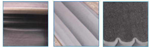
Heat-weldable TPR sidesheets (left) integrate with the deck waterproofing system. Silicone bellows provide a watertight top surface (center) of Emshield UL/ULC fire-rated foam. The top and bottom of each foam stick is coated with traffic-grade silicone (right).
