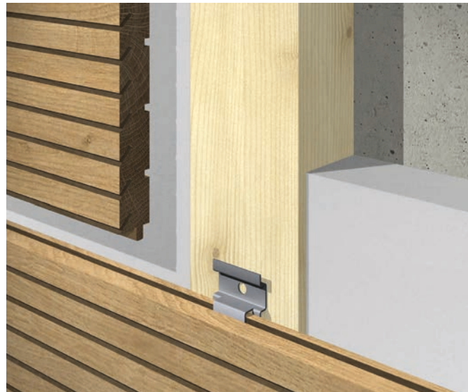
detailed view: horizontal mounting with mounting clip
