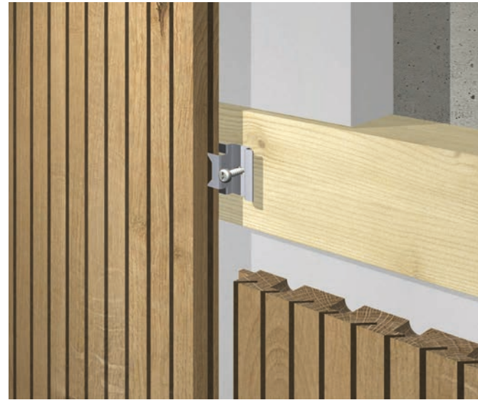
detailed view: vertical mounting with mounting clip
