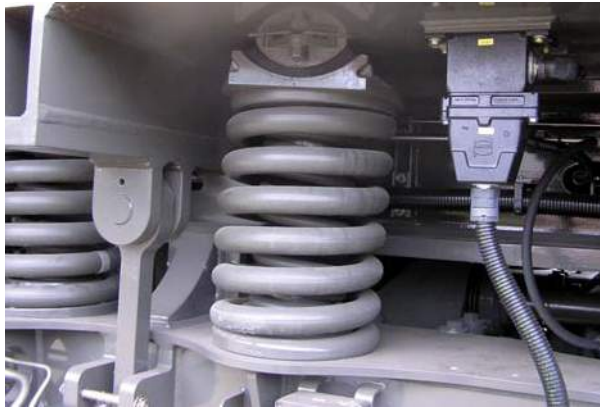
Frame support with rubber on top of steel spring.
