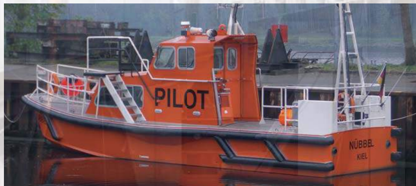
Individually manufactured fender strip of PE foam with PUR skin
