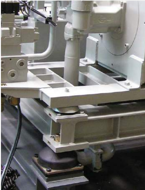
Double elastic vibration mount for industrial machine
