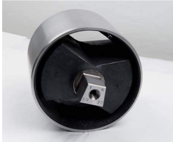
Axle guiding bush for housing (Görlitz 8 DD)
