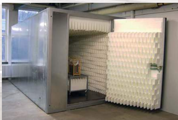
Soundproof test room made with Contrabel
