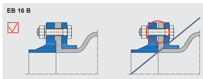
When using loose flanges with thick bead, the gap above the bolts between both flanges must be filled with an appropriate ring. This stops the loose flange from tilting and thus prevents incorrect contact with the sealing surface!
