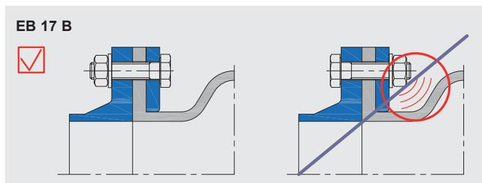
**Exception:** If the expansion joint has a long collar (supporting shoulder), the bolt can also be inserted the other way round - however the bolt must not be longer than the collar!
