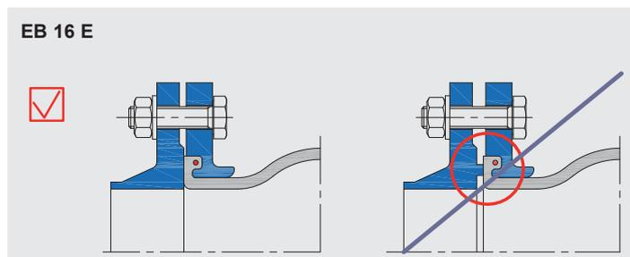
Ensure during fitting that the rubber bead is located correctly in the groove of the expansion joint flange, otherwise the sealing surface may be damaged and leaks can occur!
