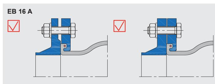
If a smooth flange cannot be used for expansion joints with solid rubber flanges, the recess of the counter flange must be compensated with a sealing with an appropriately thick ring or taken into account in rubber flange fabrication.
