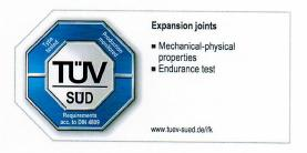
The product satisfies the requirements based on the DIN 4809 "Expansion joints made of elastomeric composite materials (rubber compensators) for water heating systems "with max.100  $^{\circ}$  C / 10 bar or with 110  $^{\circ}$  c / 6 bar.
