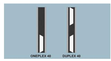
**ONEPLEX 40** is a combi blade designed for medium and heavy ploughs. It is mostly used on Vario ploughs where ordinary rubber blades are not strong enough.
