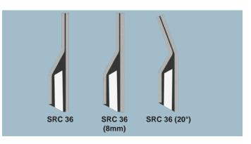
**SRC 36, SRC 36 (8mm) and SRC 36 (20°)** are combi blades designed for medium and heavy ploughs. The thickness is ideal, giving less resistance, allowing fast driving and yet remaining efficient. These universal blades are the best replacement for classic steel blades due to a longer lifespan. Not recommended for sensitive surfaces or on roads with signal markings. SRC 36 (8mm) has a stronger 8mm front plate. SRC 36 (20°) is a special version of the 8mm with an additional 20° angle.
