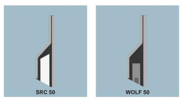
**SRC 50** is a combi blade designed for medium and heavy ploughs. The thickness is ideal giving less resistance, allowing fast driving and yet remaining efficient. This universal blade is the best replacement for classic steel blades due to a longer lifespan. This is the longest lasting blade with corundum segments. Not recommended for sensitive surfaces or roads with signal markings.
