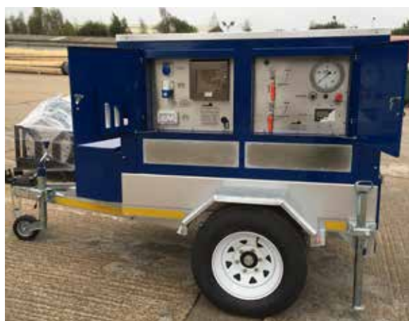
Hose testing equipment
