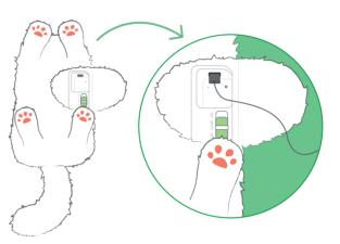
Charge your metacat with a type-c cable and you will see the blue light when successfully connected
