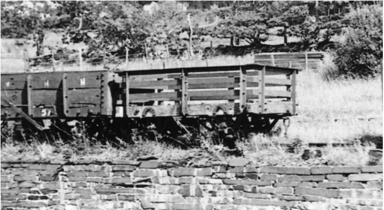
Photo 4) - One of the ex-NWNGR 'Iron Crate' slate wagons photographed at Dinas Junction after the closure of the Welsh Highland. A number of key features are readily identifiable in this image although the level of detail discernible below the solebars is disappointing - H.C. Casserley - 18 th July 1941.
