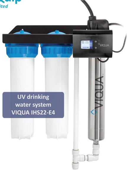
**WaterQuip's Viqua IHS22-E4** is a professional line high-capacity fully integrated water purification system that cleans water using proven ultraviolet (UV) disinfection technology and fine sediment and taste/odour filters. UV is a chemical free process which deactivates bacteria, virus, and protozoa by up to 99.99%, thus providing clean and safe drinking water which meets the World Health Organization's and local health departments' standards for potable water.
