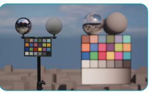
The diffuse and specular chrome balls are used together to provide a complete picture of the lighting conditions in a scene. By using both types of chrome balls, filmmakers can ensure that the lighting in their final shots will be consistent, even if different shots were captured at different times or in different locations.
