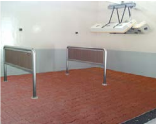
Figure 3: Pressure load for simulation of lying down (joint calotte).
