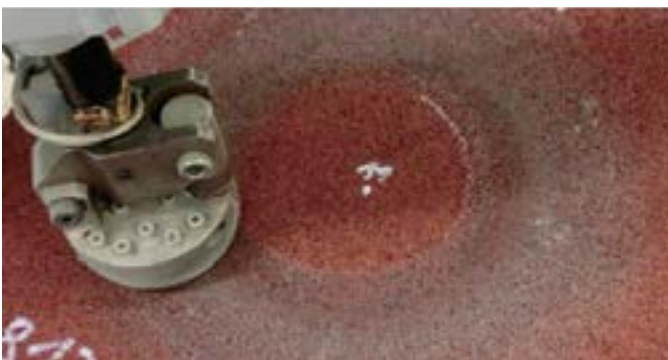
Figure 4: Pressure load for simulation of active movement (horseshoe).
