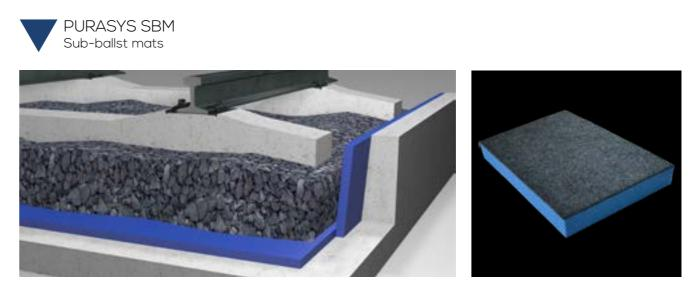
PURASYS SBM products are decoupling and protective mats under rail systems tested according to DIN 45673-5 (Mechanical vibration - Elastic elements of the superstructure of railway tracks). They reduce structure-borne noise and secondary airborne sound as well as vibration emissions. For ballasted tracks, the service life is extended by a lower and more even load. At the same time, it can protect engineering structures or sealings.
