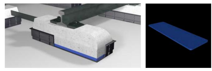
PURASYS ESB products are individually prefabricated, elastic inserts for sleeper boots. This enables different sinking values to be compensated for. At the same time, they serve to optimize load distribution and reduce the forces that occur. By decoupling the track from the ground, PURASYS ESB also achieves greater drive comfort.
