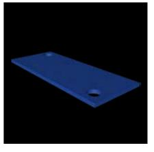
PURASYS BPP products are intermediate plates that increase the elasticity of the rail superstructure. The rails are decoupled from the ground and the high dynamic forces acting on the rail, fastening system and pavement are reduced.
