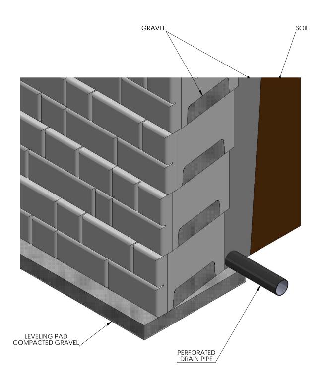
DRAIN PIPE IS PLACED BEHIND THE BLOCK AND ON TOP OF THE LEVENING PAD. THIS OPTION REQUIRES 1' OF LOOSE GRAVEL BEHIND THE WALL.
