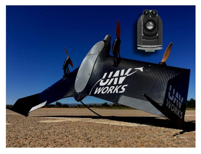
In addition, integrated NextVision's *Colibri 2* gyrostabilized x40 visual and x4 thermal camera captures high-resolution images and records and streams HD video with automatic object tracking capability, adding invaluable data in high demanding missions.
