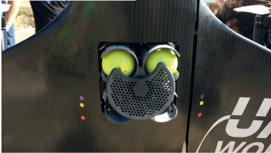
The VALAQ 120's payload dispenser in the aircraft's belly was loaded with golf balls as test substitutes for the forest fire re-ignition sensors tried out in the Ethon firefighting project
