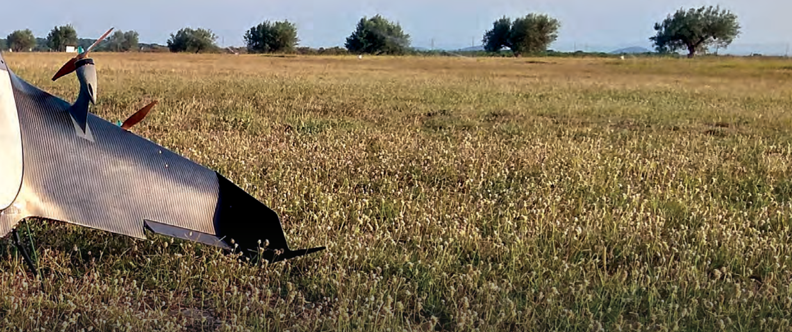
The VALAQ 120 ready to launch, sitting on its three-point landing gear. The two elevons, one on each wing, are the only moving control surfaces (Images courtesy of UAV Works)
