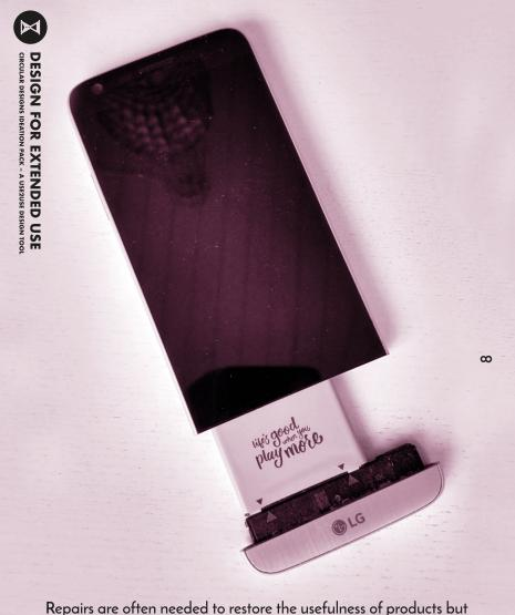
can be tricky for people to carry out by themselves. The mobile phone LG G5 is a good example of a product designed for ease of restoration when the battery is worn out. It only takes the user a minute to change the battery, with no tools needed.
