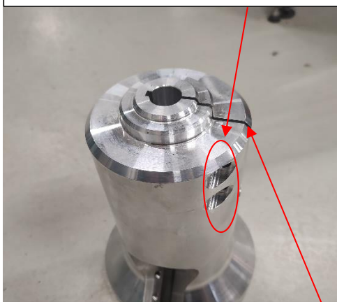
Crack that can be fitted with a wedge
