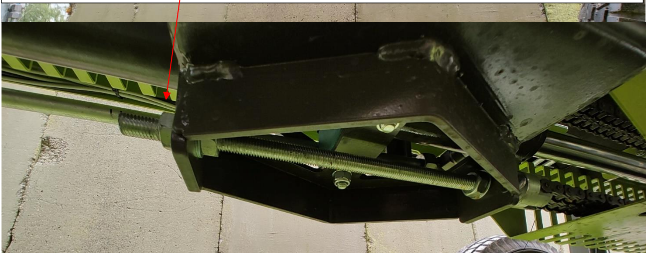
Nuts loosening threaded rod Nut for chain tensioning
