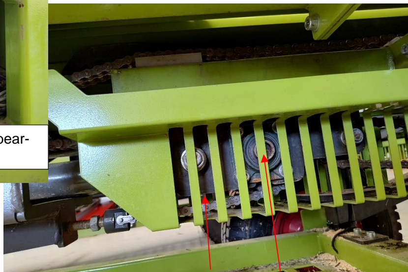
Lubrication points exchange, 1X pivot bearing, 2X bearings
