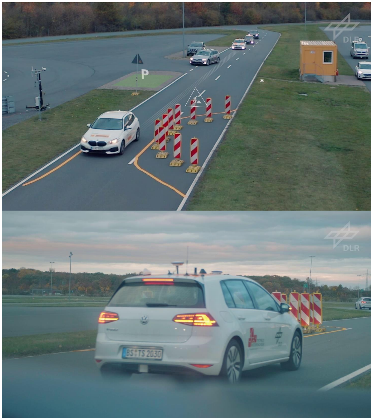
Figure 7: ViewCar2 enters available safe-spot (top) upon I2V message reception. FASCarE needs to stop on the road as no safe-spot is available (bottom).
