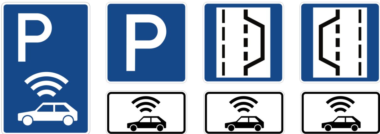
Figure 39: Static signs for parking restrictions (based on German signs 314 and 315, left) and safe spots (right, based on German sign 324, M4)
