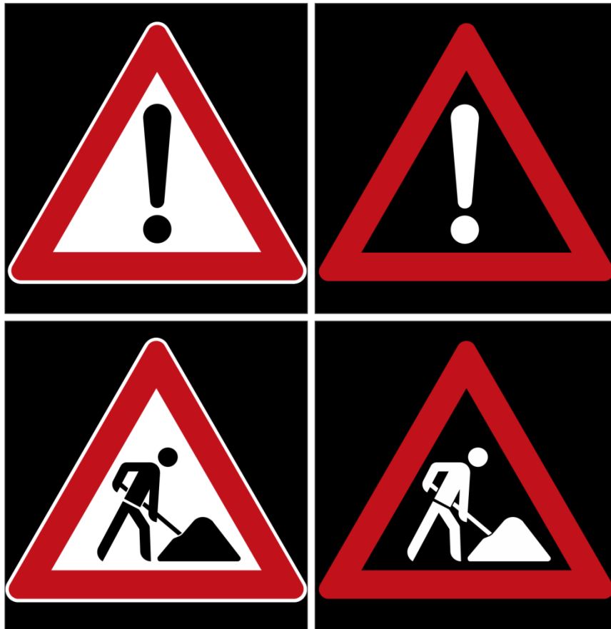
Figure 33: VMS designs for areas which need to be handled with attention, unspecified (based on German sign 101, above) and special case example roadworks (based on German sign 123, below) (R4)
