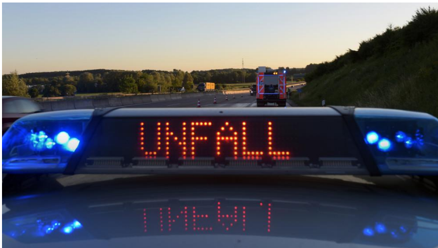
Figure 22: Rooftop light bar with a complex display on a German emergency vehicle (Source: dpa)
