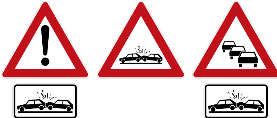
Figure 35: Static signs warning about possible collisions due to any reason (based on German signs 101, 124 and 1006-31, C1, C2, C3)
