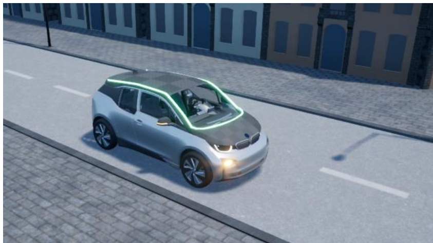
Figure 21: An external LED strip used for communication to VRUs in the project interACT [41]
