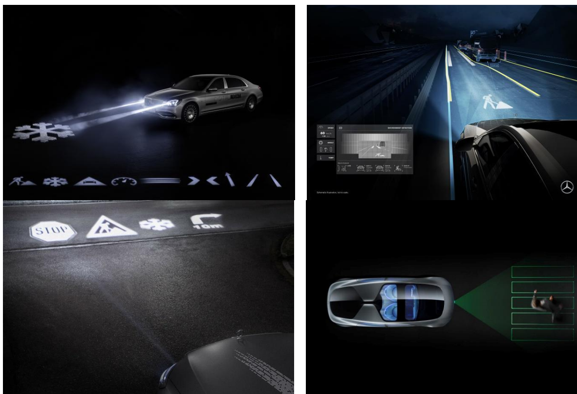
Figure 26: Daimler's Digital Light concept and the F 015 laser projection system (Source: "Mercedes News" Forum, [44])
