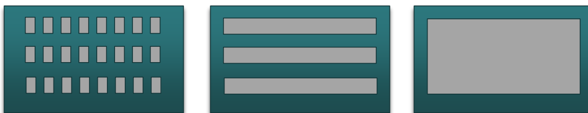
Figure 15: Variable Message Sign Matrix Displays: Character Matrix, Line Matrix and Full Matrix (from left to right)
