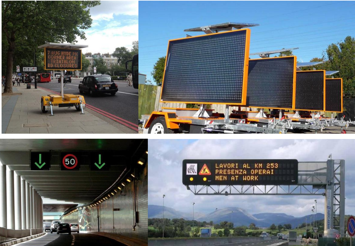
Figure 16: Variable Message Signs examples (Above: mobile trailer versions; Below: Overheads versions)
