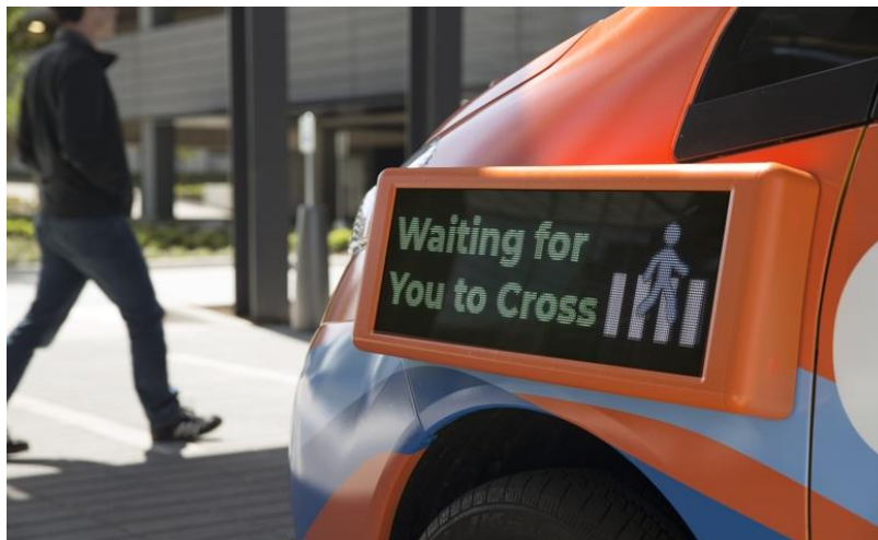
Figure 24: Drive.AI pioneered the use of an external LED-display screen that can convey a self-driving car's intentions to humans. (Drive.AI [43])
