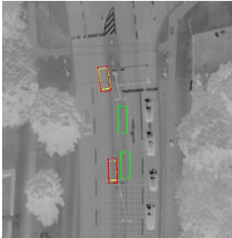
Figure 40: Fusion result (red boxes) between lidar (yellow boxes) and CPM (green boxes)
