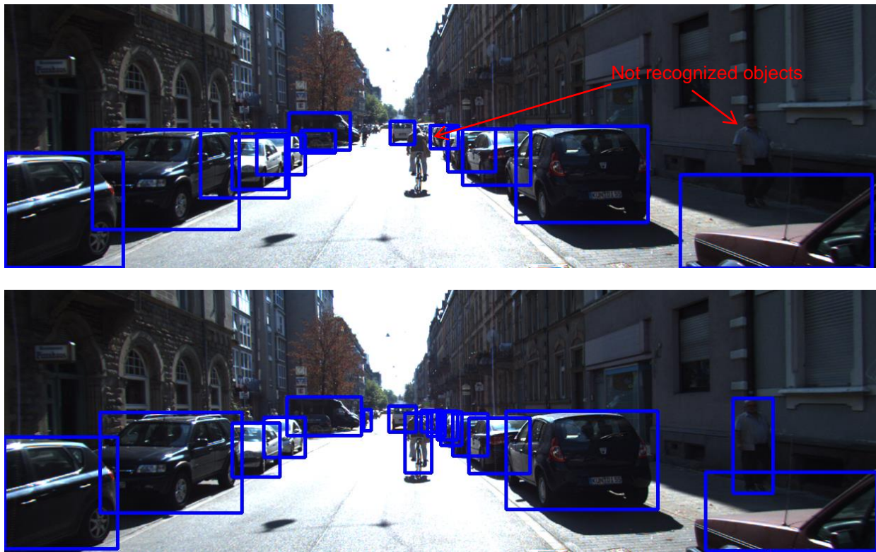
Figure 15. CNN-based detection result with backbone MobileNetV1 (upper image) and with backbone ResNet 101 (lower image). Image source: KITTI dataset [39].
