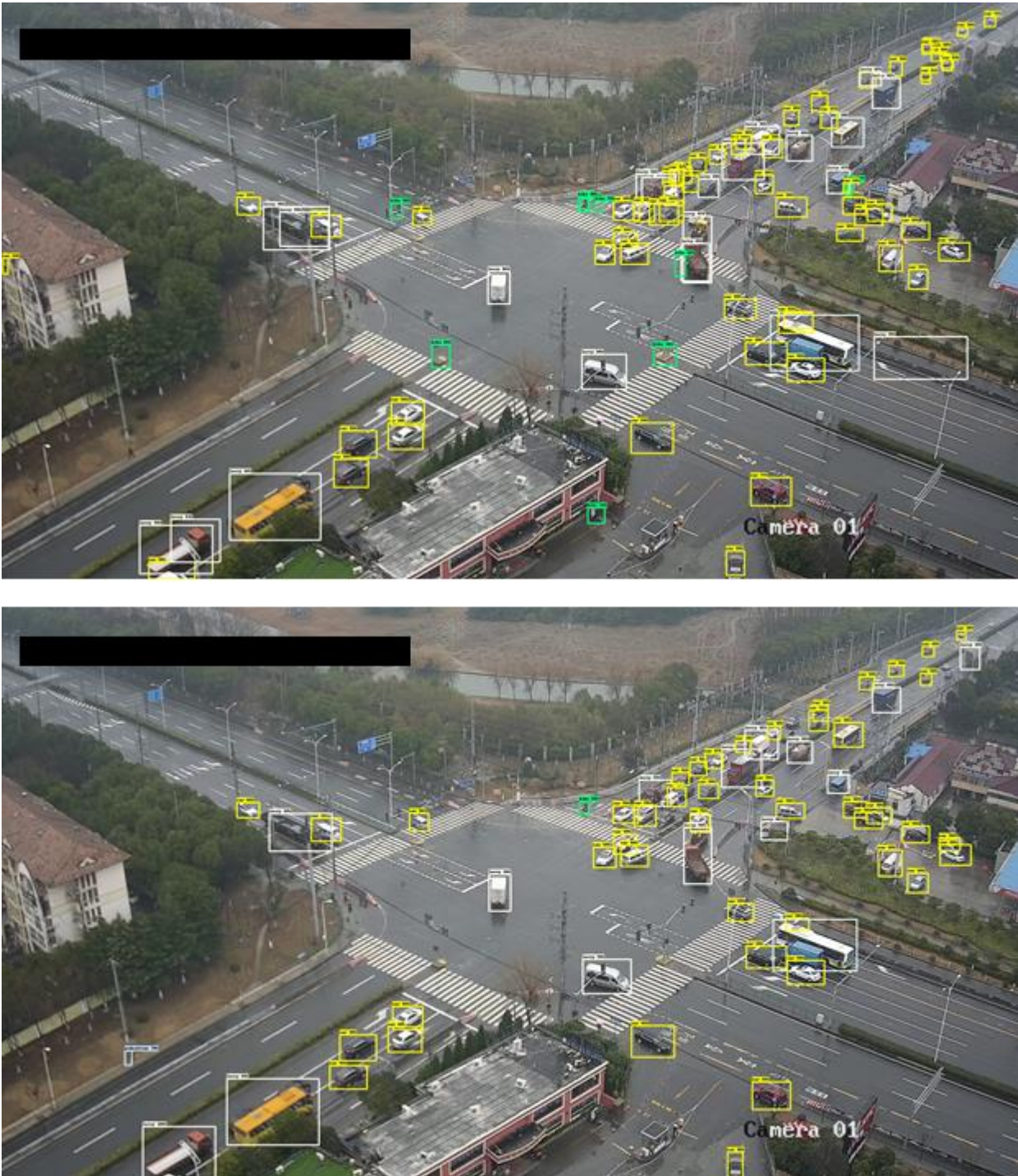
Figure 34: Result of the detection with a Faster R-CNN before (upper image) and after (lower image) the fine-tuning on the additionally labeled dataset
