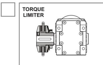
If the application is with high shock loads and sudden stops it's suggested to use mechanical or electronic torque limiting devices.
