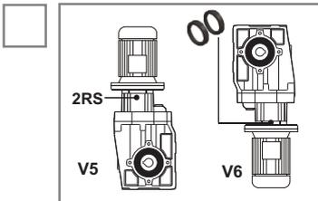
Please specify when ordering if reducer are used in Vertical V5 or V6 mounting position. We normally mount a 2RS self lubricated bearings ( see picture ) for V6 mounting we recommend double oil seals in the input side V6 positions is not recommended for 2 poles motors
