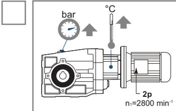
High speed motors, Higher than 1800 rpm, can produce high operating temperatures within the reducer and should only be used for intermittent duty applications. Decrease the reducer's lubricant levels and install a breather plug.
