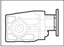
**4** Selection tables can be used also for the mounting version P (With IEC B5 - B14 motor flange ).
