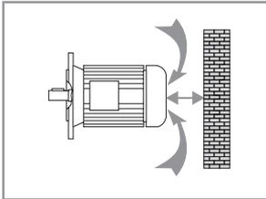
Make sure there is sufficient space between any obstructions and the motor's air intake area to provide adequate cooling for the motor.
