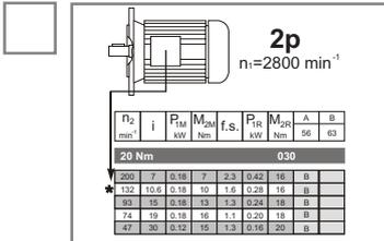
With 2 poles motor if a particular " low noise" is required ask us the most suitable ratio.
