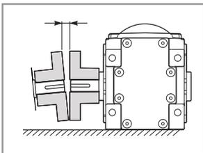
Check shaft and coupling alignment. Check proper coupling gap before to lock all foundation bolts that should be routinely checked.
