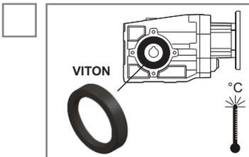
In case of high temperatures we suggest to use FPM (fkm) Oil seals in the output shaft.
