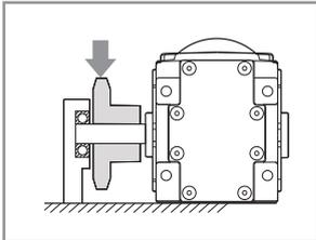
For very heavy radial load, additional output shaft support may be required to prevent premature bearing failure or shaft breakage from bending fatigue.
