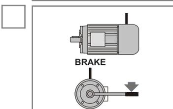
Reducers are not to be considered fail safe or self-locking devices. If these features are required, a properly sized, independent holding device should be used. Reducers should not be used as a brake. Any brakes that are used in conjunction with a reducer must be sized or positioned in such a way so as to not subject the reducer to loads beyond the catalog rating.
