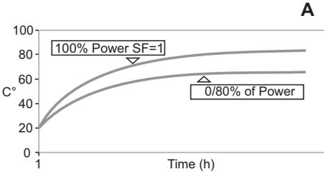
Worm gearboxes, because of their inside design, transform part of their installed power into heat which is subsequently disposed of throughout the housing and may result into values, measured onto the gear case in the area of the worm shaft, in the range of 80 - 100 °C without this affecting the operation of the gear unit adversely.
