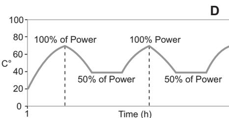
**Geared motor selections with 2800 min<sup>-1</sup> input speed are tolerated for intermittent duty applications only, because of the high temperature in crease resulting from the input rotation speed.**
