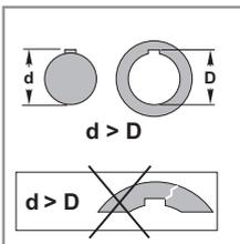
When mounting items to the reducer shaft, appropriate anti-seize and oxidizer compounds should be used, and keys dimensions are correct.
