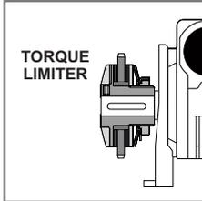
If the application is with high shock loads and sudden stops it's suggested to use mechanical or electronic torque limiting devices.
