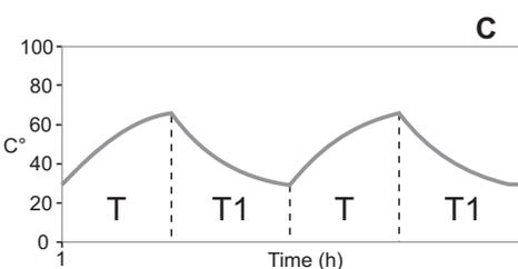
Should the gearbox have several starts and stops cycles, the final temperature depends on starts and stops times (very similar to electric motors with operation S3 and S6 see graphs C and D).
