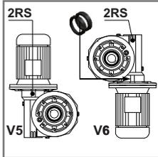
Please specify when ordering if reducer are used in Vertical V5 or V6 mounting position. We normally mount a 2RS self lubricated bearings ( see picture ) for V6 mounting we recommend double oil seals in the input side V6 positions is not recommended for 2 poles motors
