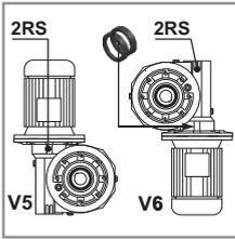
Do not change mounting positions without contacting our factory. Altering the mounting position may require special lubrication provisions which must be installed from the factory. When reducers are mounted in positions V5 or V6 and used in continuous duty applications, replace the upper bearing with a self lubricated style bearing, and we suggest double input seal for V6.
