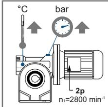
High speed motors, Higher than 1800 rpm, can produce high operating temperatures within the reducer and should only be used for intermittent duty applications. Decrease the reducer's lubricant levels and install a breather plug.
