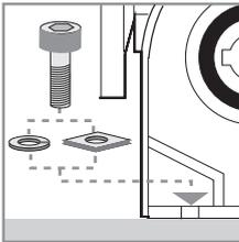
Mount the reducer on a flat surface free of vibration. If high over hung loads are expected, it is advisable to reinforced bolt heads with washers as shown in picture.
