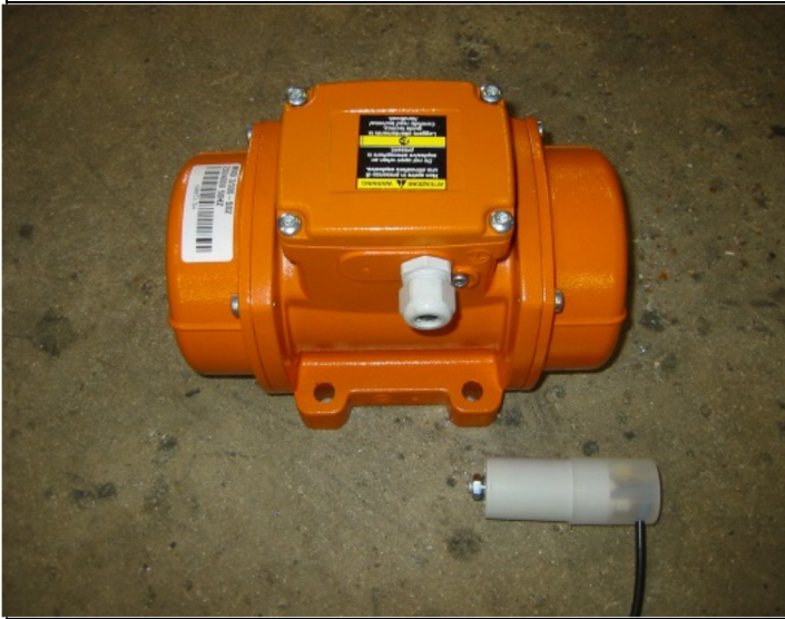
Vibrator with loose Capacitor (s) No cable
