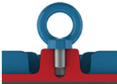
Figure 4.1 - Correct tightening of the eyebolt
