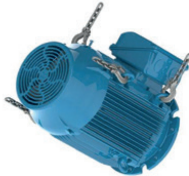
Figure 4.18 - Motor is being rotated to horizontal position
