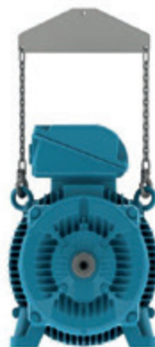
Figure 4.6 - Use of a spreader beam for lifting
