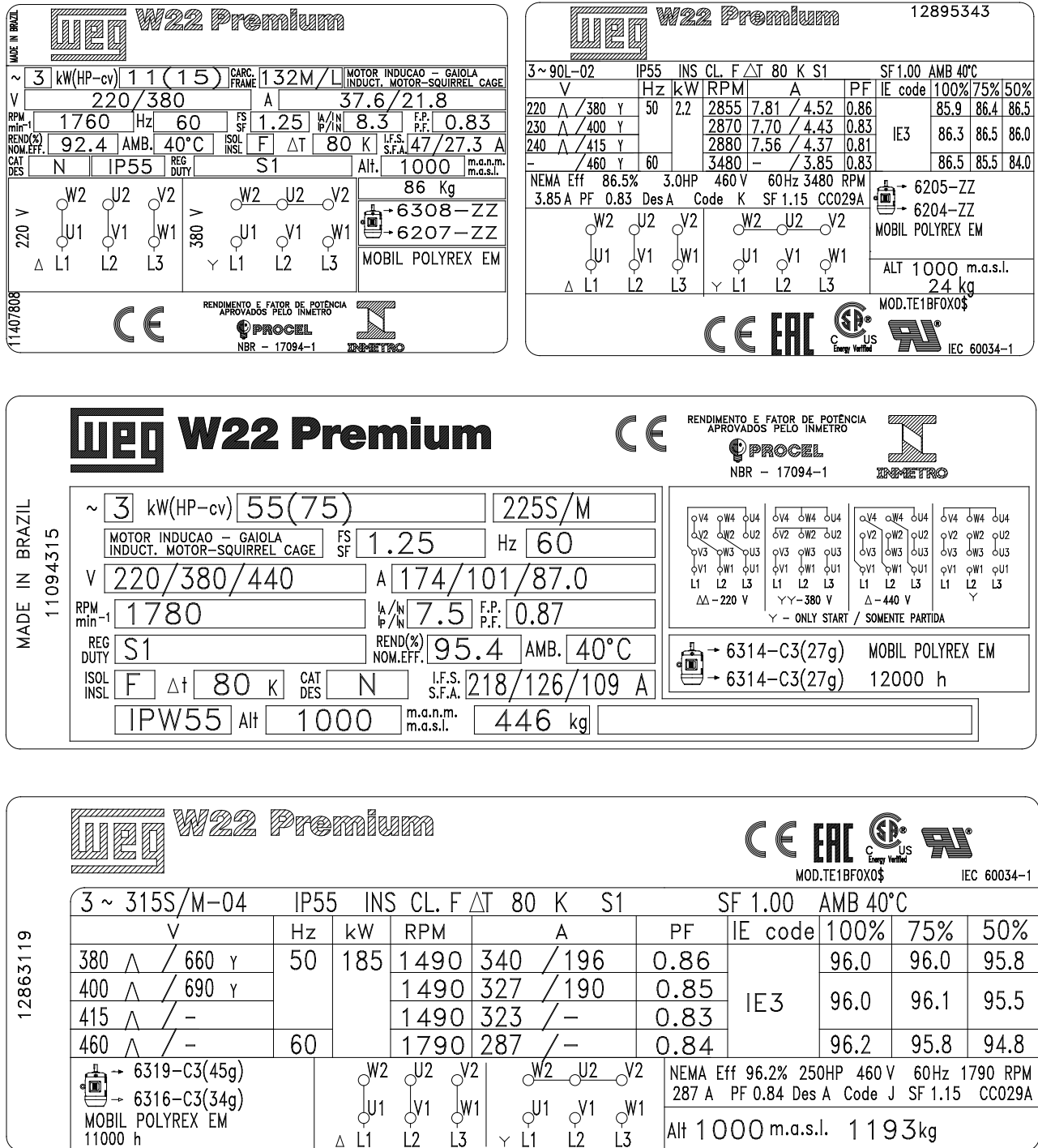
Figure 2.1 - IEC motor nameplate
