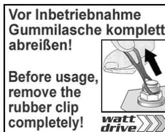
Fig. 2: Information label (red) on the gear unit
