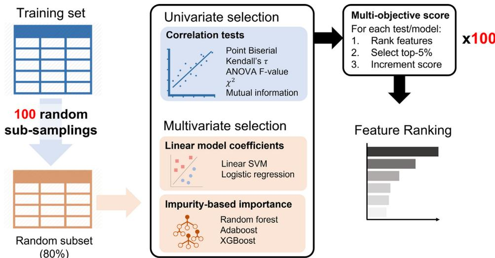
Fig. 8. Diagram showing the our multi-objective feature ranking pipeline, combining the respective strengths of filter and embedded approaches to features selection. Abbreviations: SVM, support vector machine.
