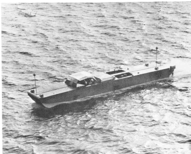
FIGURE 6 - Characteristics of high length/beam ratio SES were determined from tests of the XR-5.
