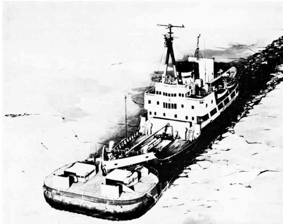
FIGURE 2 Bell Aerospace artist's impression of ACV bow fitted to Icebreaker CCGS Montcalm
