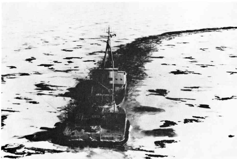
FIGURE 13 CCGS Alexander Henry with ACT-100 (Iceater I). Note the ice is broken along the side of the ship giving a wider effective track than with a ship operating alone.
