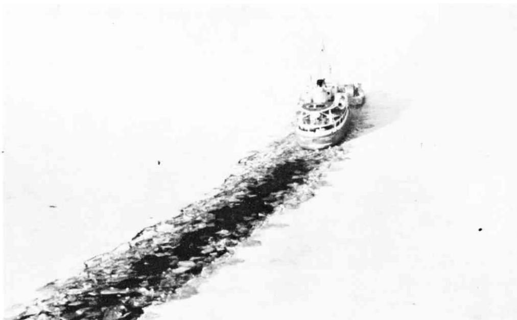
FIGURE 11 Track broken with air cushion platform attached to Alexander Henry - operating in ice 37-42 cms (14-16 ins) thick
