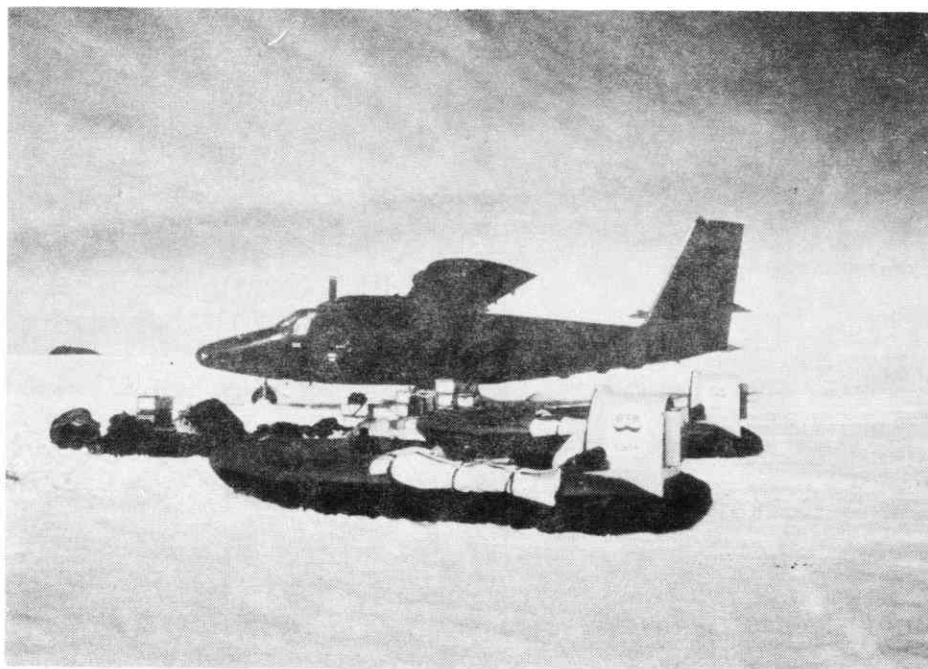
Air Vehicles "Tiger 4" , United Kingdom Dim.: 5.1m by 2.4m, Load: 325kg, Max. W.: 550 kg
