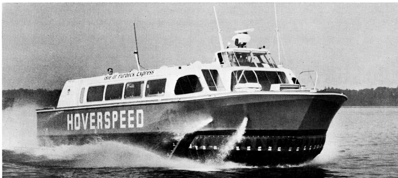
HM-2, 60 seater, 35 kt. sidewall type hovercraft. Powered by marine diesel engines. Positive directional control. Quiet in operation. Low capital cost. Low operating costs.
