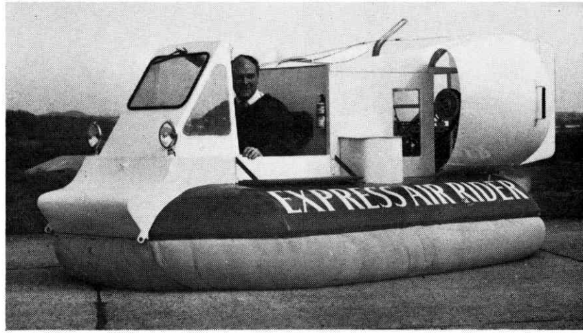
November 6th, 1966. The first public demonstration (above left) of the first Express Air Rider. (Above right) The original Air Rider after considerable modifications including the addition of about 60 lb. of glass-fibre, elaborate ducting of the propellers, and the addition of a small bow shape and a new windscreen with wiper. Even headlamps were fitted. In this form the craft proved to be far too heavy and much of the extra weight, including most of the glass-fibre, was stripped away.
