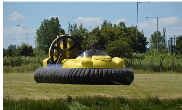
Above, the BHC Coastal Pro with separate lift and thrust motors.
