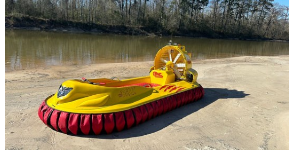
The BHC Beast XL with Briggs and Stratton V twin 4 stroke power, integrated lift and thrust.
