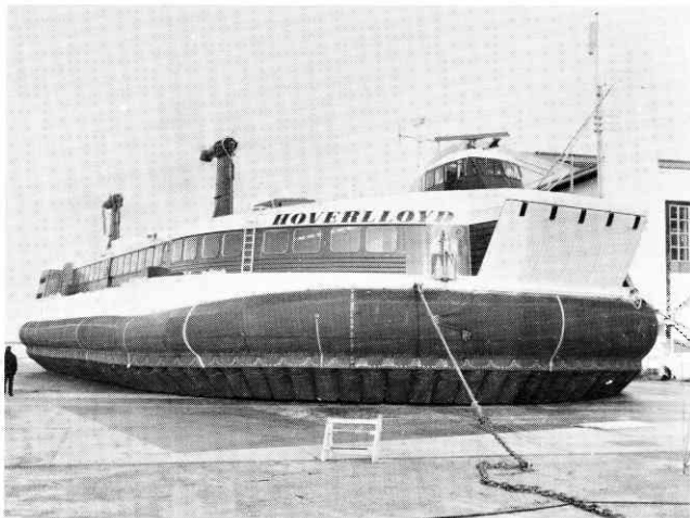
FIG.10 SR.N4 Mk.1 LATER CRAFT FITTED WITH Mk.2 SKIRT – DEEP BOW
