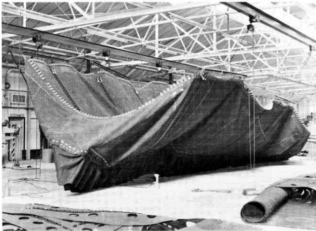
FIG.19 VIEW OF REAR SKIRT BAG AND CONES, SUSPENDED IN SKIRT SHOP DURING MANUFACTURE
