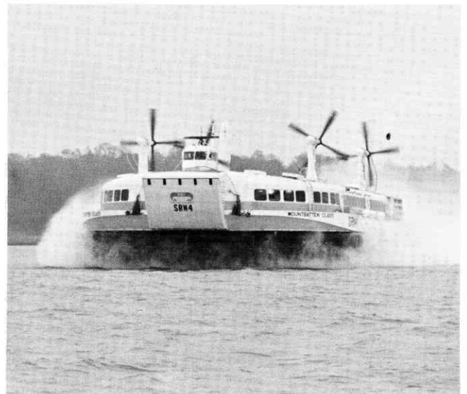
FIG.9 SR.N4 Mk.1 PROTOTYPE – SHOWING Mk.1 SKIRT WITH SHALLOW BOW
