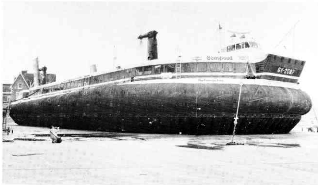
FIG. 15 FIRST SUPER-4 (GH.2007) DURING INITIAL TETHERED HOVER TESTS
