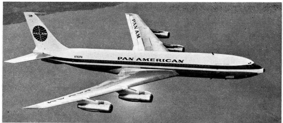
Right, a Boeing 707-320B jetliner; below, the French Line flagship "France." Respective work-capacities are 10,560 ton-kt and 11,200 ton-kt; yet the liner costs ten times as much and weighs some 400 times as much
