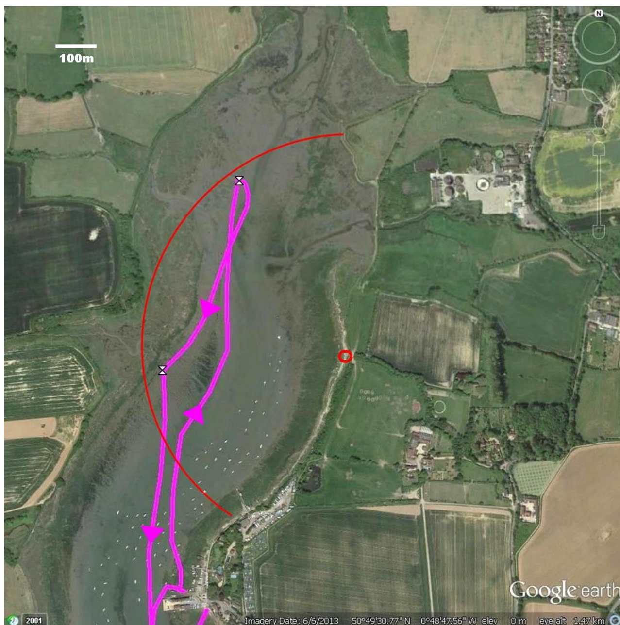
Map H: Track taken by hovercraft at Dell Quay including sample points as measured using Garmin eTrex GPS
