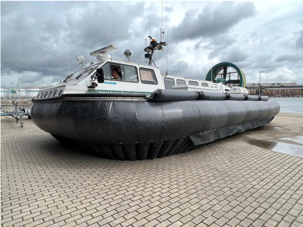
This 2000TD hovercraft, built in 2000, has just been fitted with a brand-new skirt system to keep it operational for at least another 5 years. The work was carried out for the customer in-country by Griffon Hoverwork Support Services Team. Photo courtesy the Lithuanian Border Guard.
